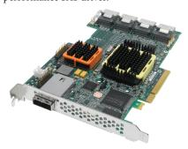
The 20-port (16 internal/4 external) Adaptec RAID 51645 utilizes industry-leading dual core RAID on Chip (ROC), 512MB of DDR2 write cache, and connectivity with the latest x8 PCI-Express to deliver over 250,000 I/Os 1.2GBs. Using SAS expanders, it can connect up to 256 SATA/SAS devices. Adaptec Intelligent Power Management slashes power and cooling costs by spinning down idle disks and providing a lower power mode for active disks.
